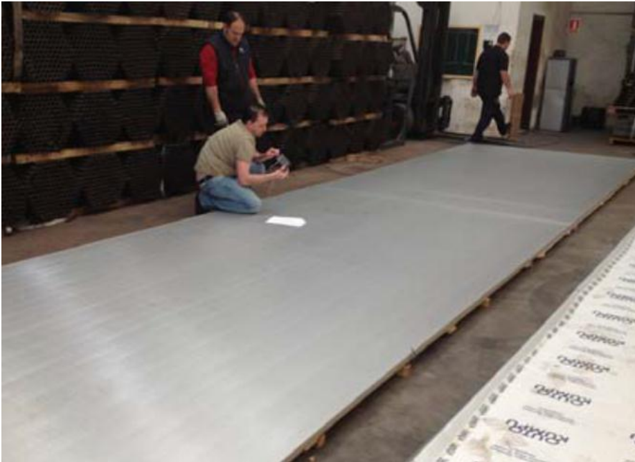
A plate of the cryostat vessel body
